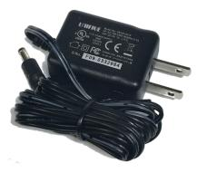
AC Adapter - Ultra mini size Inp: 100-240VAC, Output: 5Vdc @1Amp DC Connector: 4.0 x 1.7 (EIAJ-2) Level 6 compliant Model: PS-1512
